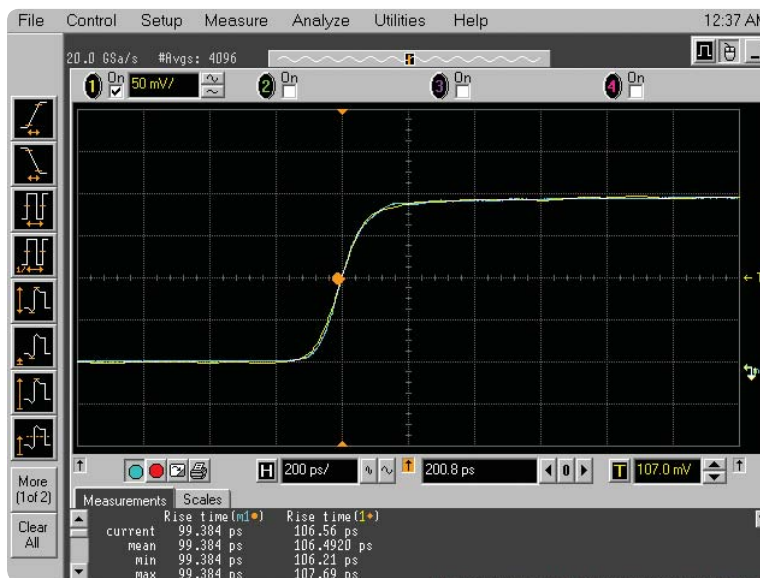
Figure 29. Response of a 54855A oscilloscope combined with an 1134A 7 GHz probe amp and an E2677A differential solder-in probe head at 100 ps
